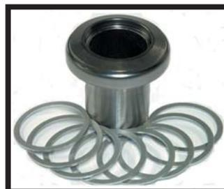
**RH7161 Extended Length Sleeve & Bearing Kit** This kit is used to convert a standard length HRB to an extended length HRB. It includes a 1/2" taller sleeve & bearing and the shims needed for extremely short clutch / tall bellhousing applications.
