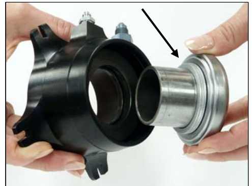
Fig. 6: Install shims over sleeve
